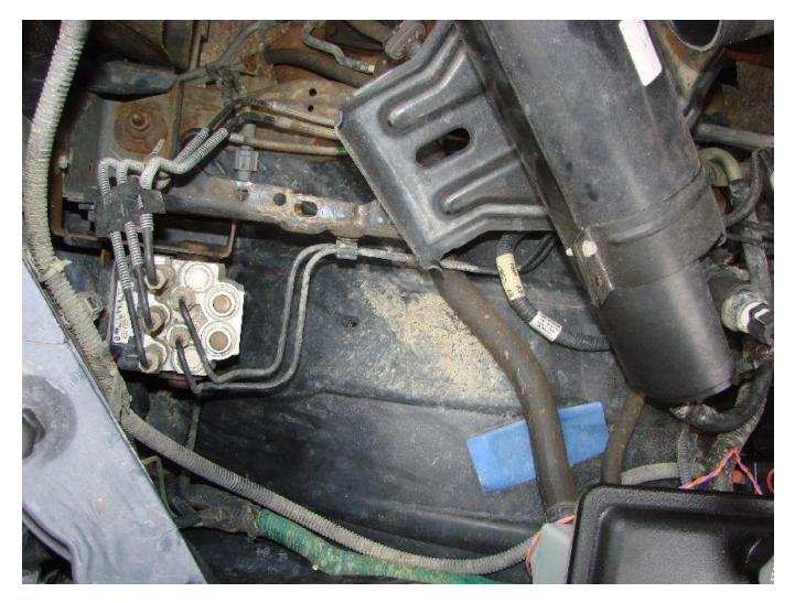
4. Instead of trying to make the necessary connection right at the abs module, it is much easier to make the splice where this wire harness is. Remove the tape (in this case green tape) surrounding the wire harness.
