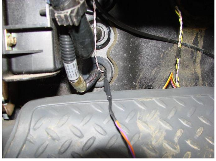
Merlin Controls Speed Wizard Detailed Install 99-04 Super Duty REV 1 3/5/08 You will notice the Violet and orange wires go through the lowest firewall rubber grommet. This is where I had the most room on my truck, however the user can use their best discretion to choose where to push the speed wizard wires through.
