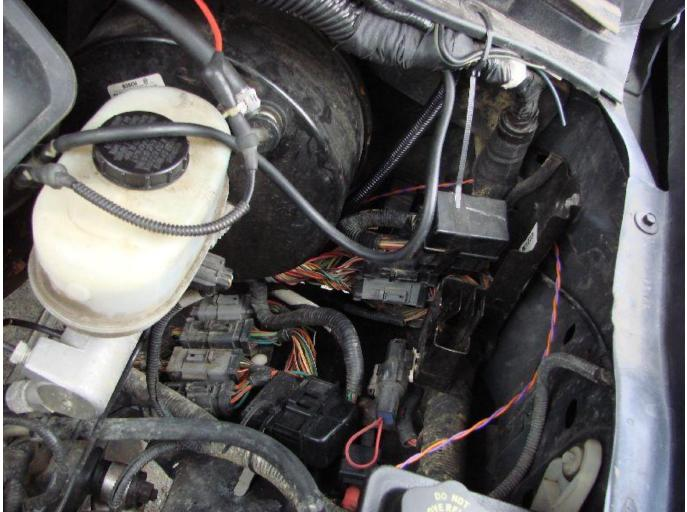
The wires go right through the firewall on the driver's side. Make sure the wires do not scrape against anything that will cut through the insulation. The user may decide to install wire loom around the wire, this is a great idea to protect the wire even more.
